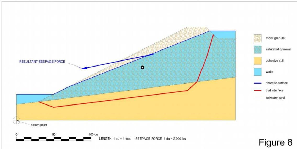
comparison with the “no pond” condition the FoS for the c&φ embankment fill drops by 41% while the reduction in stability for the fully frictional material is far greater, at 56%.
